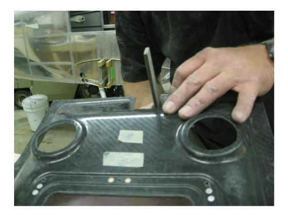
To begin fitting, you will want to find and mark the center points of your cabin top. You will want to do this at the bulkhead as well as at the front. Also, mark the centerline of your console at the front and back. You can do this by marking the centerline on a piece of masking tape. The first trimming of the console will usually occur at the step or jog located directly aft of the doors. If needed, you will trim the console down here to allow it to drop down and sit flush on the cabin.
