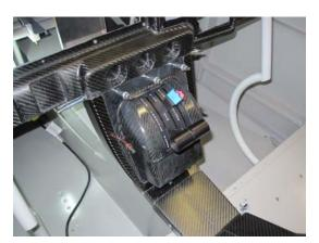
In the best of situations you are installing the lower console of the instrument panel and the center arm rest console at the same time. Once the flange is cut off, you will need to ensure that the lower console panel and the center arm rest console mate perfectly flush with each other. Align the top so that it smooth. Since there is a gap to slide carpet underneath each side there is some lateral movement. Just align both pieces so the gap is equal on both sides of the tunnel.
