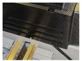
Using a strap duplicator, locate and drill the holes on the tunnel covers. A #19 strap duplicator works well, but you will want to enlarge the holes with a #12 drill bit afterwards. Also, you don't have to use every hole in the tunnel cover to mount the arm rest. It is recommended using at least four holes.
