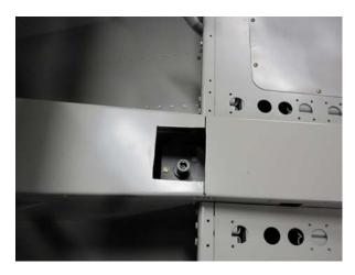
Additionally, it is suggested that you may want to cut your tunnel cover into two pieces. This will allow greater convenience for performing conditional inspections. You can see in the photo to the left there is a natural break just at the front edge of the front seats. There are also two screws located close together so additional screw holes aren't required.
