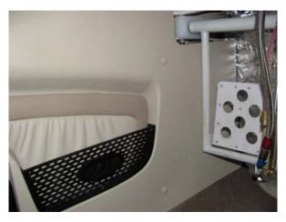
These dimensions are not critical but should be close. Use 6-32 screws and K-1000-06 nut plates.
