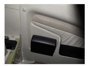
The Lower hole is not critical as to location but should be just above landing gear support bar so you can get drill this hole and insert #6 self tapping sheet metal screw. Be sure that there are no conduit, wiring, or tubing located in proximity to this location.
