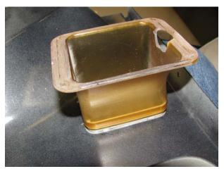
Test fit the panels with the vents installed. Carefully install the vent cover into your side panel and snap the panel edge over the snaps on the vent cover. Once complete carefully push the deflector tube over the vent cover. This is a tight fit so please be patient. You may need to sand the deflector tube a little bit to get the fit. Try to keep the deflector tube square to the vent cover when trying to fit everything together.
